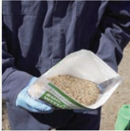
2 Sprinkle the sawdust mixture (Package 1) over the contaminated area
